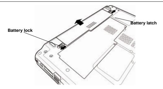
Figure 4-1 Removing the battery pack
